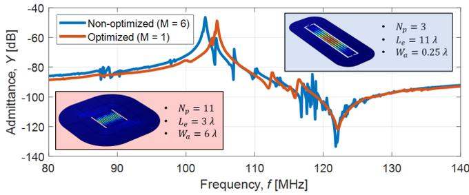
Fig. 7. COMSOL® 3D simulations of a device with optimized significant features as predicted by the NN ( $N_p$ ,  $L_e$ , and  $W_a$ ) versus a non-optimized device. Both the number of in-band spurious and their excursion are significantly reduced. Fixed parameters:  $\lambda = 56 \mu\text{m}$ ,  $h = 1 \text{ mm}$ ,  $L_g = L_b = 0.75 \lambda$ ,  $W_a = 0.75 \lambda$ , and  $c = 0.3$ .
