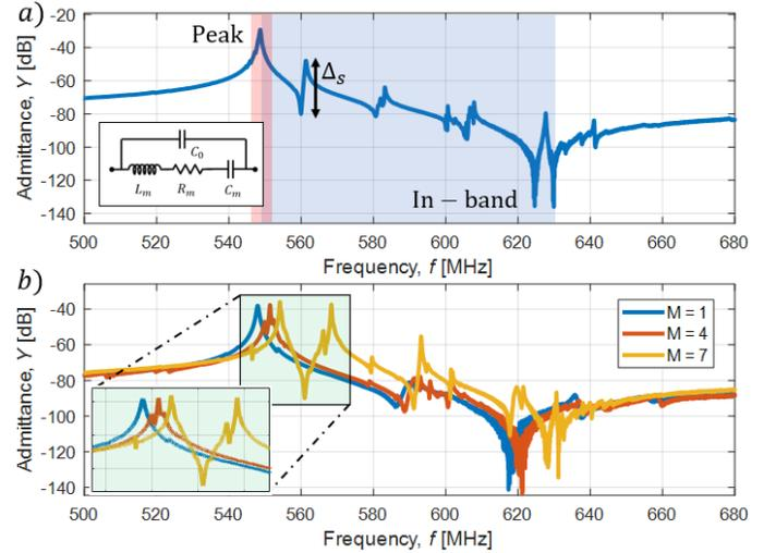
Fig. 3. a) Example of a measured LN MEMS resonator  $Y$  response. Peak and in-band regions are highlighted together with the maximum spurious peak-to-peak excursion ( $\Delta_s$ ). The equivalent electrical Butterworth-Van Dyke (BVD) model of a resonator is reported in the inset; and b) Example of device with different spurious modes  $M$  as defined in Table 2 and inset of the peak region.
