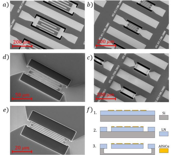
Fig. 2. SEM images of fabricated devices operating at: a) 100 MHz; b) 200 MHz; c) 400 MHz; d) 550 MHz; e) 1 GHz; and f) LN resonators fabrication process [3]: (1) Sputtering and etching of 300 nm of AlSiCu to define the top electrode; (2) Ion milling of the piezoelectric layer; and (3) Isotropic XeF<sub>2</sub> release.
