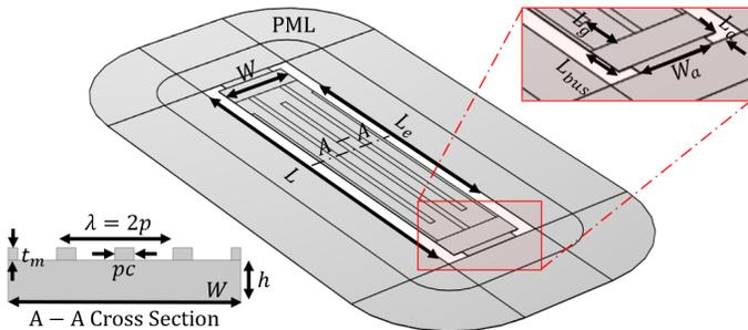
Fig. 1. COMSOL@ 2D and 3D models of a LN laterally vibrating resonators. The investigated geometrical features are highlighted in the picture and consist of: 1) Acoustic wavelength ( $\lambda$ ); 2) Number of electrode (IDEs) pairs ( $N_p$ ); 3) Electrode length ( $L_e$ ); 4) Finger-to-bus gap ( $L_g$ ); 5) Bus length ( $L_b$ ); 6) Anchor width ( $W_a$ ); 7) Film thickness ( $h$ ); and 8) Electrode coverage ( $c$ ). Boundary conditions are set via Perfectly Matched Layers (PML).
